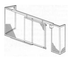
assembly except it functions in the horizontal direction and requires considerable storage room on one side when open. Another disadvantage of this type of gate is that it requires an overhead track above the gate opening.
