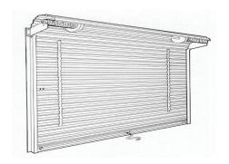
itself does not require a lot of space. Some disadvantages are that it is slow in operation, may require considerable maintenance, and it is mounted over the gate opening and may limit the load height. It may be of the manual or powered variety.
